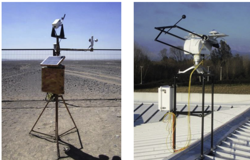
Fig. 2. RSBR station in Crucero (left) and one station with tracker, pyrhemometer and pyranometers in Talca (right).
