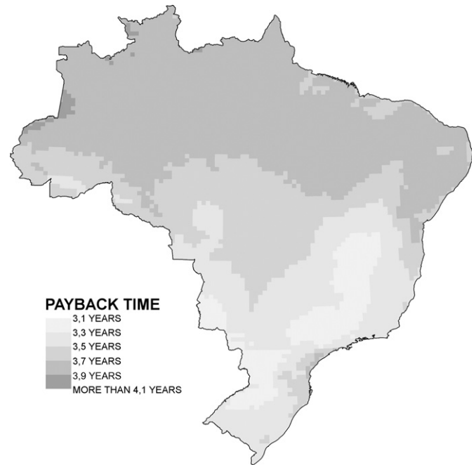
Fig. 3. Payback time for water heating by a compact low cost solar system designed to replace the electric shower in household of low-income families. Source: Pereira et al. (2008).
