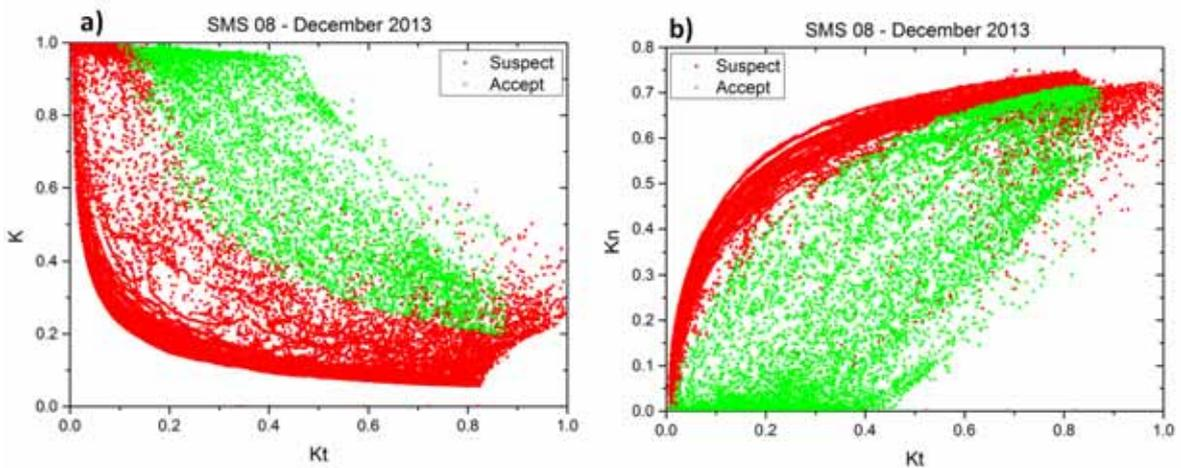
Fig. 7: Preliminary results provided by QC algorithm performed for data files acquired at São Martinho da Serra (08) to a)  $K$  vs.  $K_t$  and b)  $K_n$  vs.  $K_t$ .
