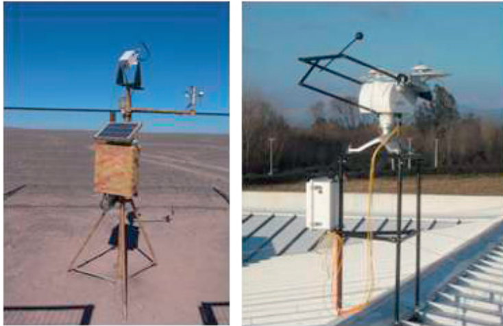
Figure 2 RSBR station in Crucero and one station with tracker, pyrheliometer, and pyranometers in Talca.
