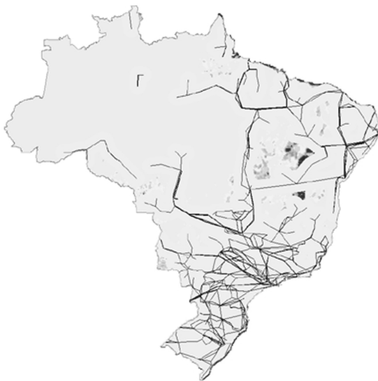
(A) (B) Fig. 4: GIS toolkit allow to make overlap energy resource maps and infra-structure information: (A) Query output showing areas with wind power density larger than 200W/m 2 and distant more than 100km far from electricity transmission lines (blue lines are the transmission lines); (B) Query output showing the Brazilian regions with solar irradiation larger than 5.5kWh/m 2 /day and distant more than 100km far from roads (green lines are the major Brazilian roads).
