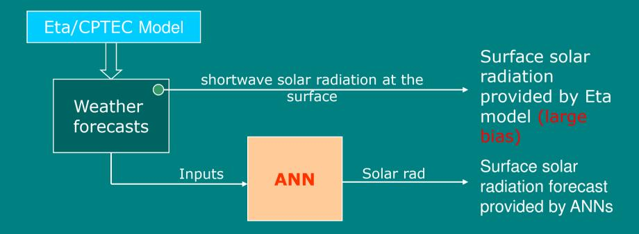
Refine the solar radiation forecasts provided by Eta model by using a statistical method based on Artificial Neural Networks (ANNs) in order to improve the reliability of the surface solar radiation forecasts supplied to energy sector.
