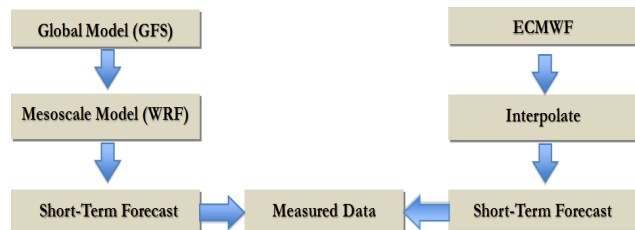
Figure 2. Schematic diagram of comparison analysis of solar irradiation forecasts provided by WRF and ECMWF models and observations at AWS.
